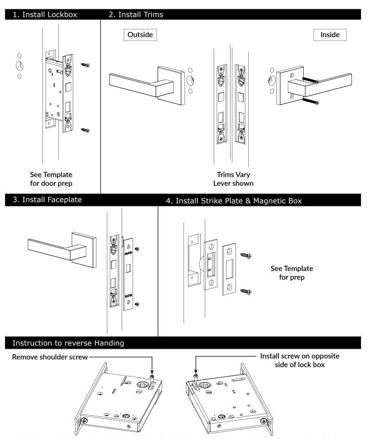
Handing can be changed to LH or RH so that the door is unlocked automatically when engaging the lever or knob from the inside. Shoulder screw should be on interior side when lock box is installed.
