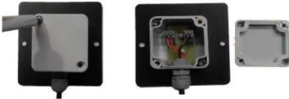
Fig. 12 – Opening the back of the wallswitch
