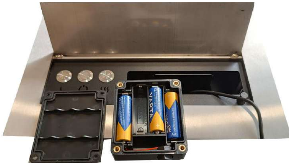
Fig. 11 – Putting back the battery box
