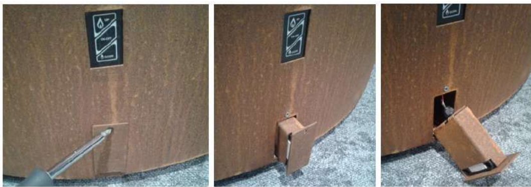
Fig. 8: Removing of the battery container
