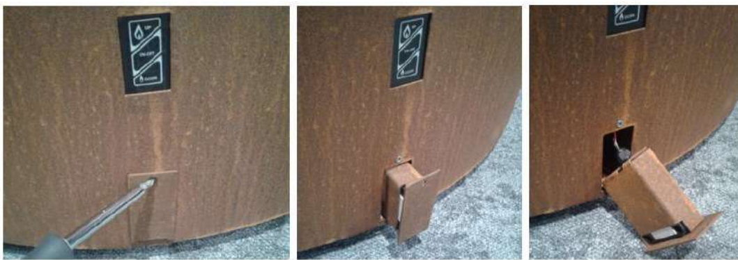
Fig. 8: Removing of the battery container
