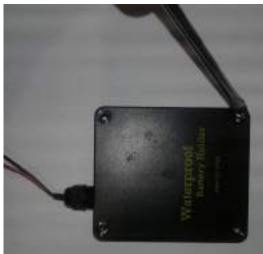
Fig 16 – Unscrewing battery box
