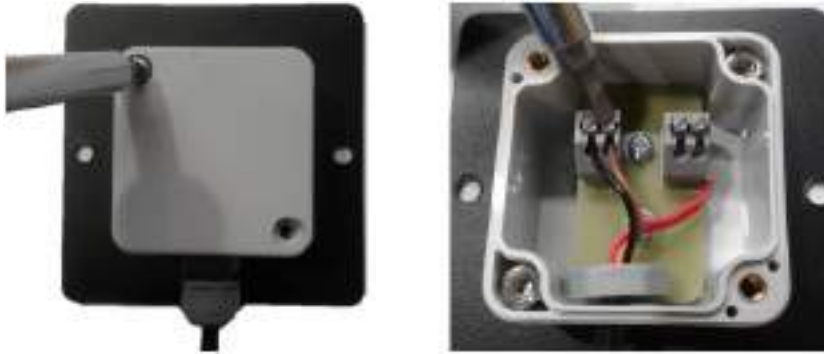
Fig. 12 – Closing the back of the wallswitch
