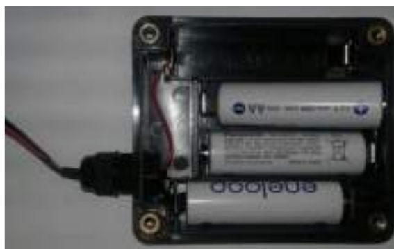
Fig 17 – Replacing battery in battery box
